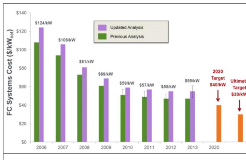
Figure 2 – Transport Fuel Cell System Cost Status and Targets, assuming a production of 500 thousand units per year. Source: U.S. Department of Energy, Office of Energy Efficiency & Renewable Energy, 2013 Fuel Cell Technologies Market Report .
